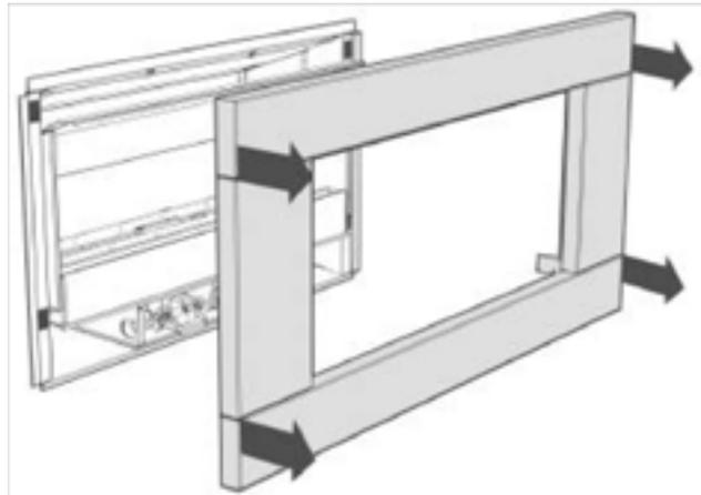
Reverse these steps to re-fit the Fascia, ensuring the two connections are correctly plugged in by testing the fire.
